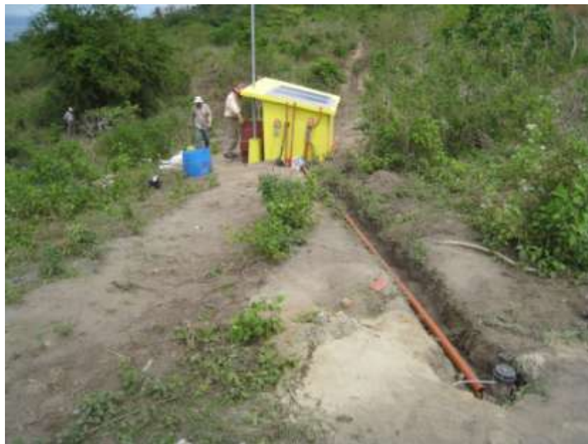
Figure 2. Installation of a continuous resistivitymeter in a Schlumberger configuration (CNRS, France) and one borehole tiltmeter (USGS, US) during March 2013 campaign.
