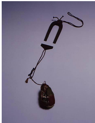
Fig.2 Horse-shoe type earthquake Indicator made by S. Sakuma
