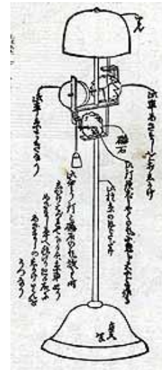
Fig.3 Magnetic seismoscope invented in Japan, as illustrated in Ansei-Kenmon-shi
