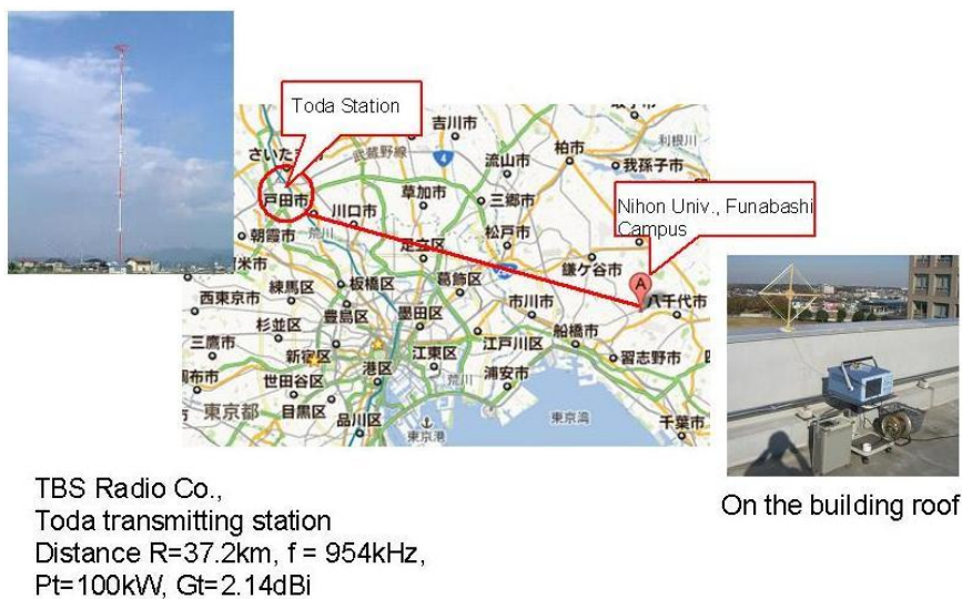
Fig.2 The locations of the transmission and reception for the calibration of the 1 MHz receiving system.
